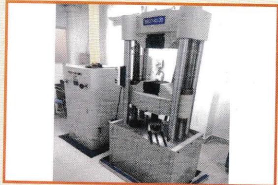
Tensile testing of weld samples in UTM
