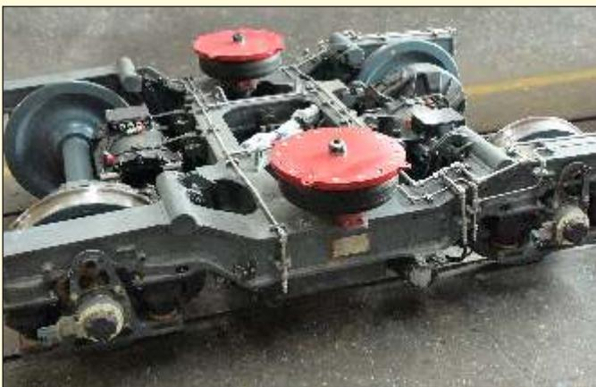
All the underslung equipment in the new metro coaches are modularized to save manufacturing/maintenance time. Regenerative braking saves the energy requirement to the extent of 30% of total consumption. Brake blending is designed in such a way that the electro pneumatic brakes smoothly take over from regenerative brake system at the fag end of braking till the train stops.
