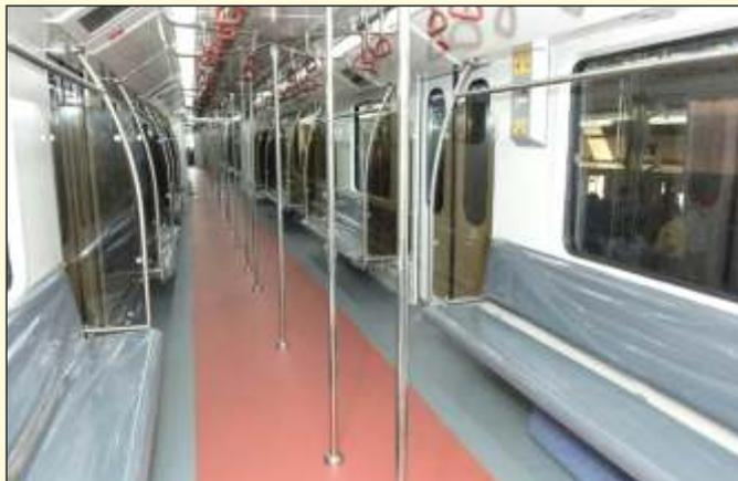
The interior furnishings are revamped to get best in class aesthetic finish. Screwless Aluminium composite panels, LED streamlined lighting, Passenger information display on LCD screens, Star grab poles, Sleek polyamide hand holds, Polycarbonate seats and Rubber twin colour flooring are some of the features of interiors.
