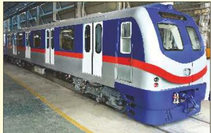
The coaches are built on stainless steel body and propelled by III-phase IGBT based electric propulsion system. The propulsion system is indigenously manufactured and supplied by M/s Medha, Hyderabad.
